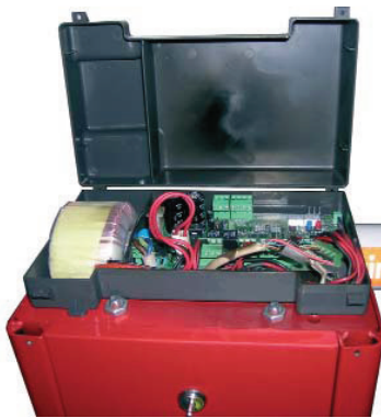
Easy access to control unit for wiring and programming.
